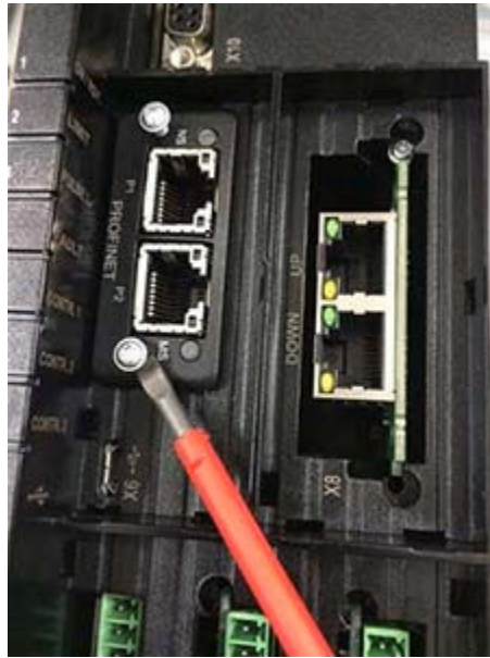
Figure 5-22. Anybus module removal
