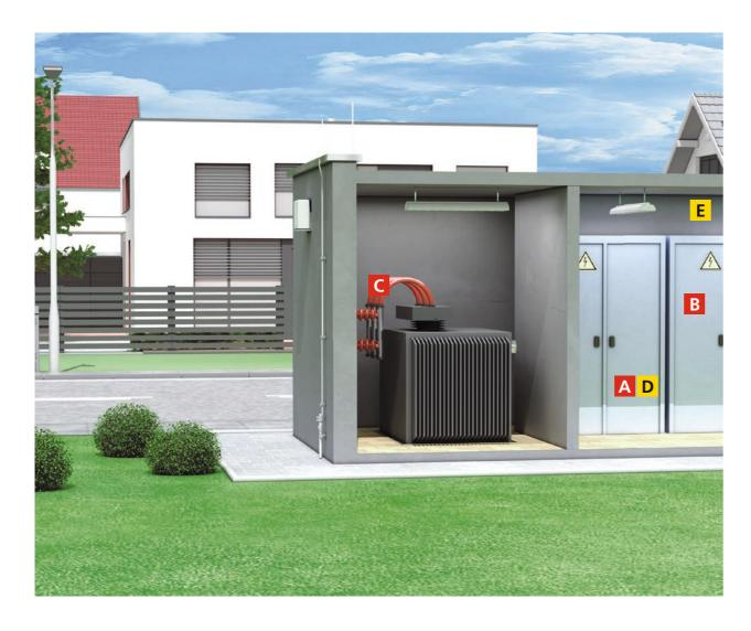
Transformer substations are an important link at the interface between medium and low voltage. If they have core components such as remotely controlled switch disconnectors and circuit breakers, regulated distribution transformers, telecontrols, communication and control devices, they are known as intelligent transformer substations.
