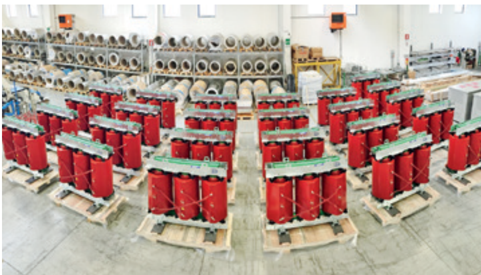
28 transformers 1.000 kVA for Gamesa Israel wind turbines
